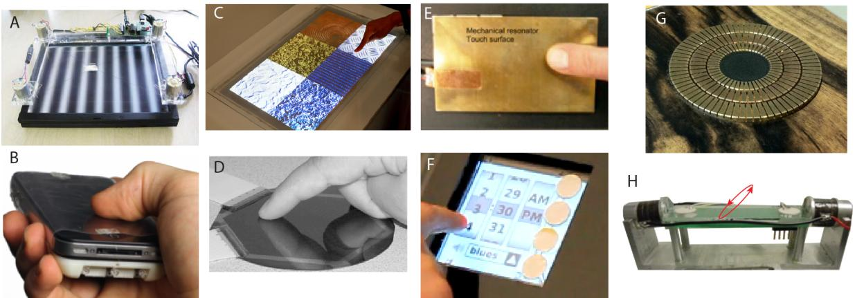
Figure 3: A. Cable-driven overlay [33]. B. Flexible wrap-around overlay [34]. C. Device using electrovibration to provide tactile texture [36]. D. Spatially distributed electrovibration device [37]. E. Ultrasonic friction modulation [41]. F. Transparent version of the ultrasonic friction modulation device. [42]. G. Travelling wave motor delivering shear forces to the static finger. H. 2-axis ultrasonic vibration delivers programmable lateral forces to the bare fingertip [46]
