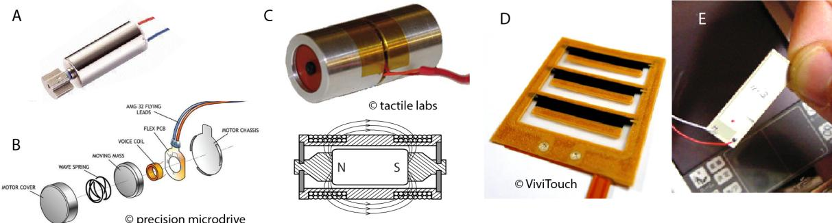
Figure 2: A. Excentric rotating motor suitable for simple rumble. B. Exploded view of a linear resonant actuator (LRA). C. The Haptuator provides a tactile stimulation with a 50 to 500 Hz frequency bandwidth using Laplace force actuation [21]. D. Example of a vibrotactile stimulator made of electroactive polymer. E. Owing to its fast response time, piezoelectric bimorph is another popular choice of material.
