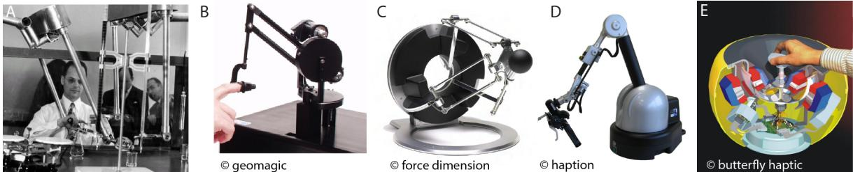
Figure 1: A. First teleoperation apparatus [5]. B. The PHANToM, one of the first commercial haptic interfaces to be developed [7]. C. Parallel robots with greater stiffness and a wider frequency bandwidth. D. Serial implementation for larger workspaces. E. Magnetic levitation replaces linkages and effectively removes friction.
