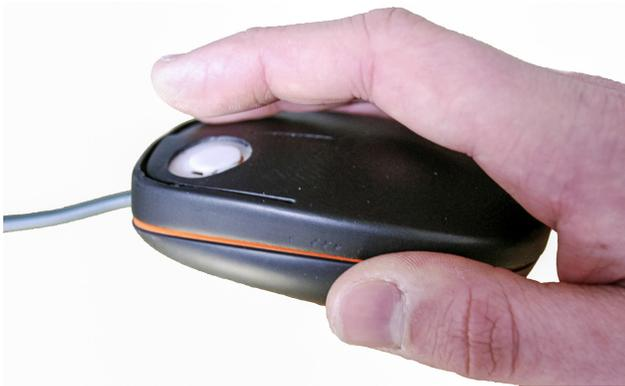
Figure 1: The *viTouch* mouse with integrated vibrotactile display.
