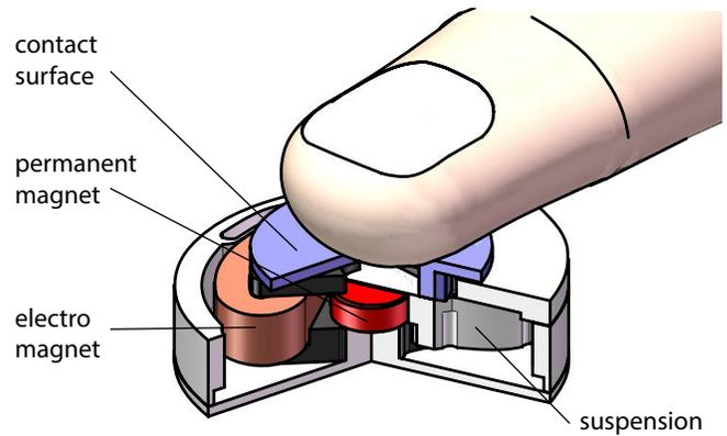
Figure 2: Cross section of the vibrotactile actuator. Electromagnetic forces applied on the permanent magnet, laterally deform the pulp of the fingertip.
