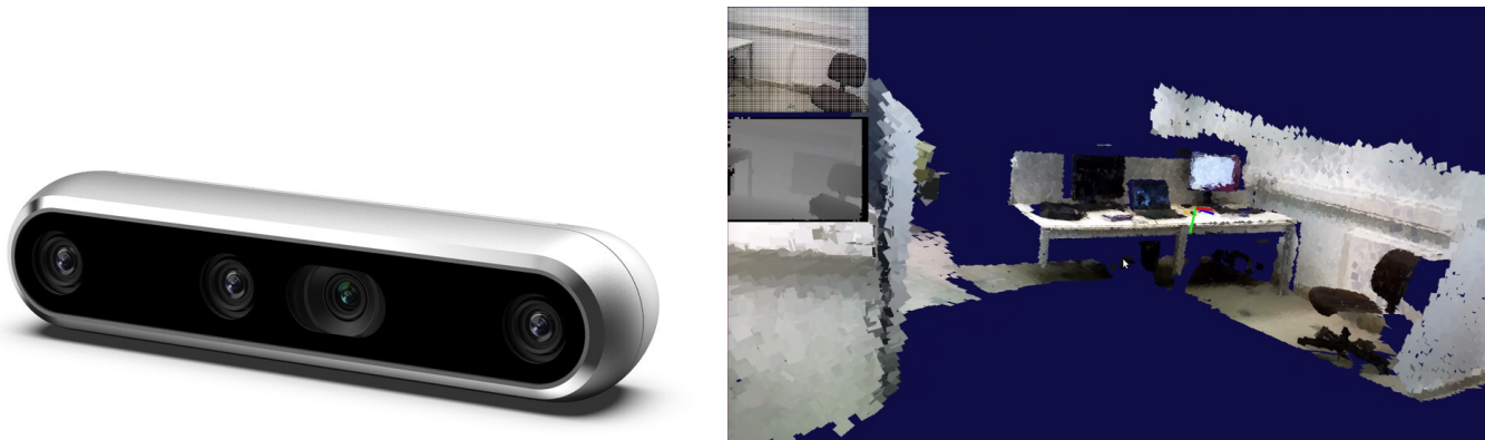
Figure 2: Left) Intel RealSense Depth Camera D455 . Right) Example of a supersurfel based reconstruction with a stereo camera.
