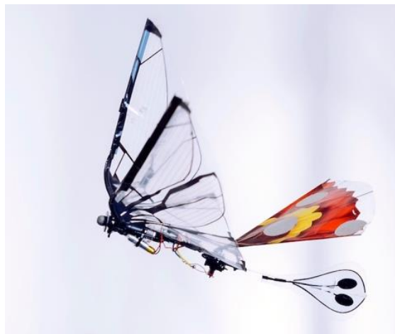
Figure 1: MetaFly (XTIM) FWUAV at the flight arena of the ISM, Marseille (Ndoye et al, IEEE ICRA 2023).
