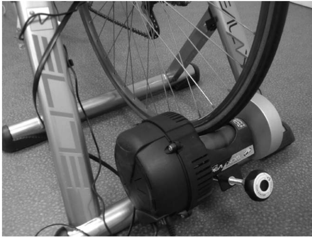
Figure 2. Electromagnetic brake and sensor placed on the bike's rear tire.
